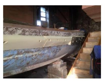
With most of the hull timber work and deck completed the team looked at ways of replicating the cork D fender towards the top of the hull. The solution indicted in the photos was to attach dense insulating foam strips to the hull and sand to the templated shape. ready for the final finish.
