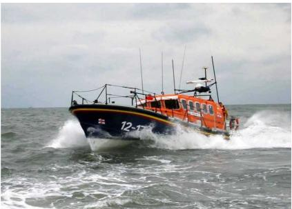
nosed bow with reverse sheer. A spray rail protects the deck and wheelhouse from thrown spray when travelling at speed. A good working space is provided on the foredeck; the reverse sheer allows clear vision over the stern when the bow rises at speed.
