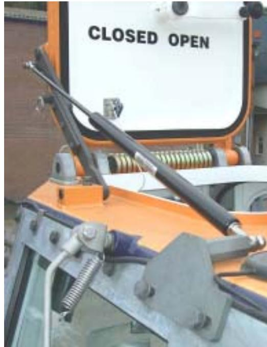
5.7.8 The hatch will close gradually and can be locked down using the catch mechanism. The inner and outer handle assemblies both perform the latching process.
