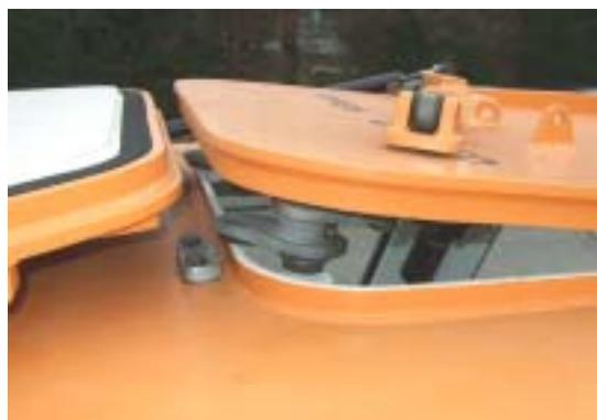
5.7.10 In the event of abandoning the tractor through the roof hatch and if time is limited, the hatch can be forced to close at a greater rate by pressing down firmly on the hatch whilst it is closing under damper control.
