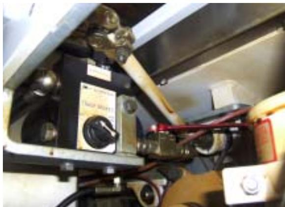
7.1.7.3 If the motors have not been bypassed, move the lever on the ball valve under cab hand pump access panel to the inline position.
