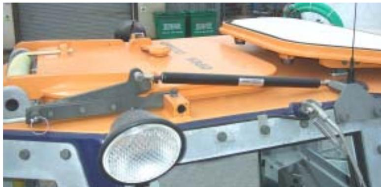
5.7.9 During normal operating conditions the roof hatch is to be set in the semi closed position with the hatch resting with the rubber catch pads on the cab roof seal rail.
