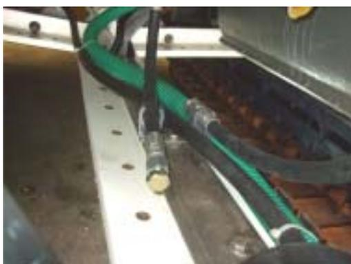
Engine sump drain & Splitter box drain
