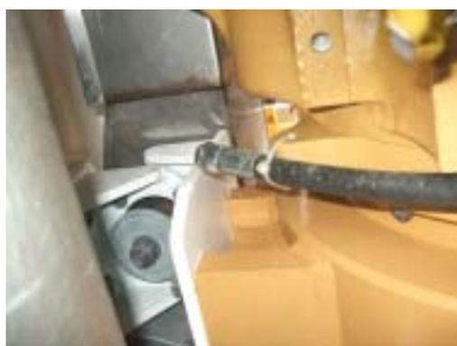
Engine block drain (coolant)
