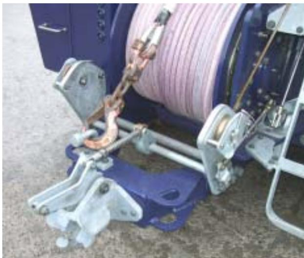
6.13.3 The handle should be returned to the parked position (away from operator), where upon re-coupling, the hook will automatically re-engage.
