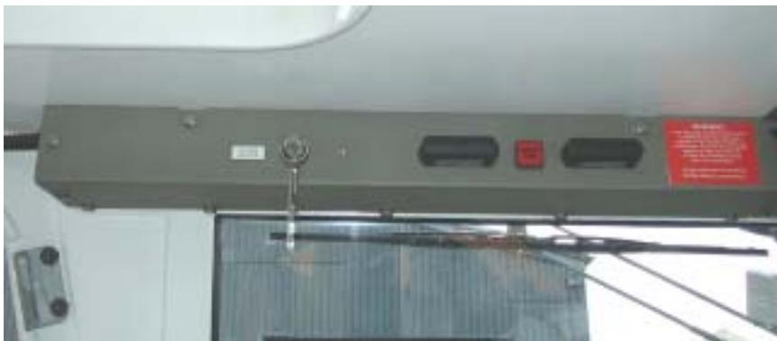
6.3.3 The push to start switch is isolated by the key switch in the rear upper panel.
